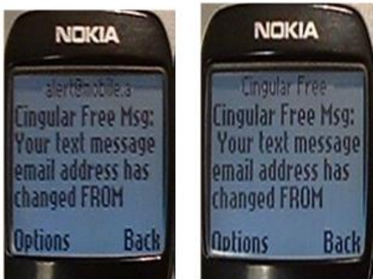
Fig 2: Spoofing a service provider notification is trivial due to interface and message length constraints; the left image is a forgery of a legitimate service notification (right) provided by Cingular (Note the top line).
